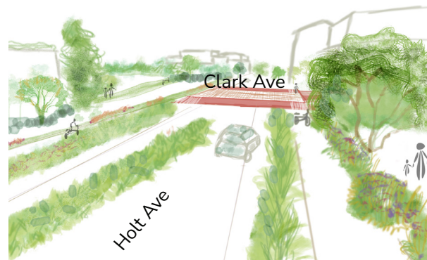
Figure 5.9 Proposed design Holt Ave, depicting median, and protected bike lanes, narrower street widths, expanded open space and increased crosswalks.
