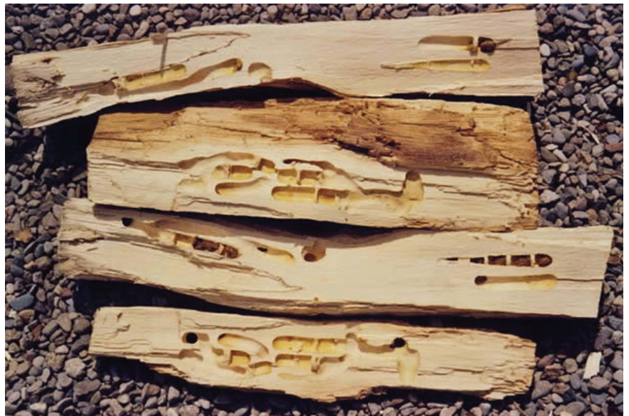
Examples of nests excavated in dead wood by Carpenter Bees. Note the cells created for the hatching of offspring, separated by partition walls. (Stephen Buchmann, USDA Forest Service)
